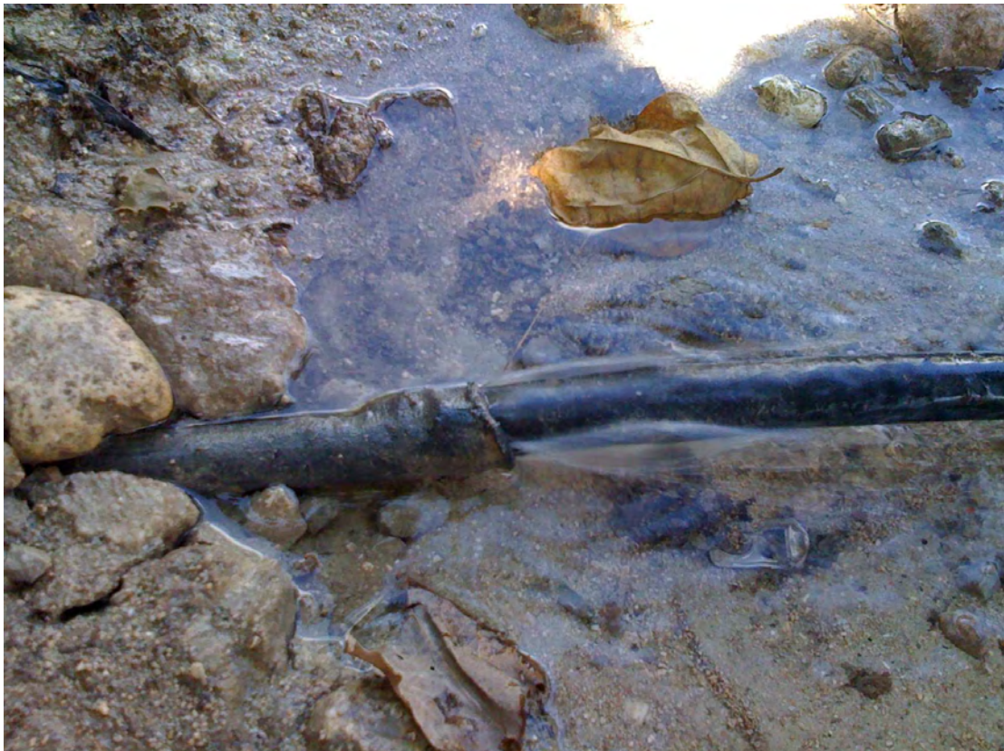
A “do it yourself” extension to get the water from the line closer to the house by forcing two pipe sections together. The only reason it didn’t blow apart was because of low system pressure. (See following photo)
